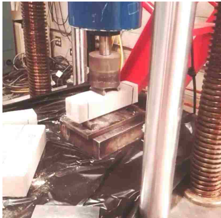
Figure 2.13. Four-Point Flexural Strength Test Set-Up
