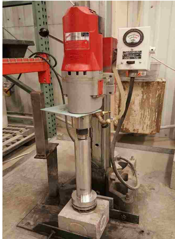
Figure 2.10: Abrasion Resistance Test Apparatus
