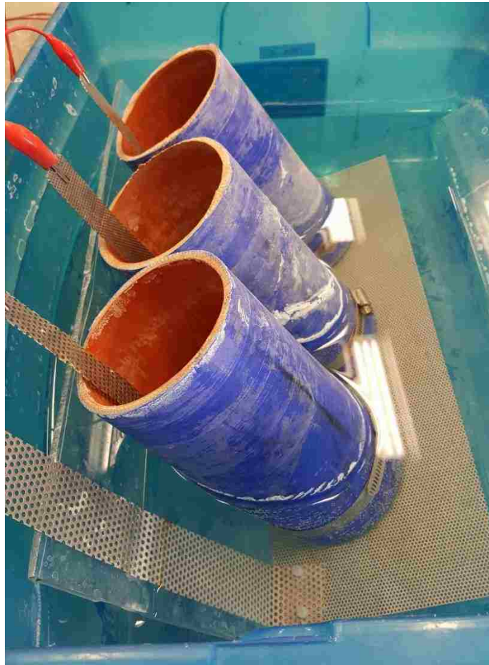
Figure 2.14. Rapid Chloride Migration Sample Test Set-Up
