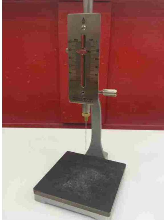
Figure 2.5. Modified Vicat Apparatus used to Measuring Setting Time
