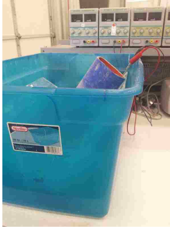
Figure 2.7. Rapid Chloride Migration Test Set-Up
